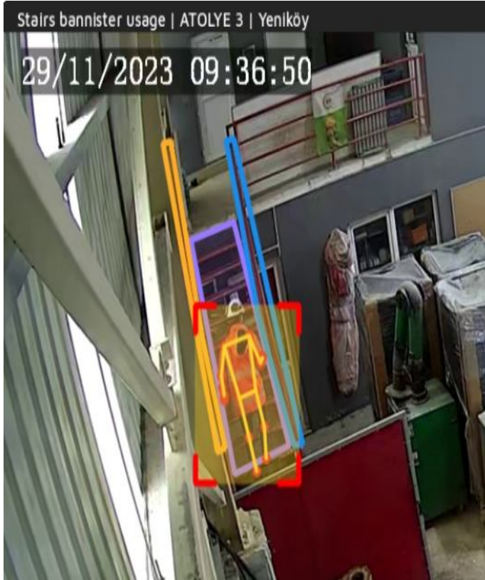
An example visual and detection of an employee not using handrails while ascending stairs.
